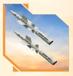
Unit (ERU) This missile is configured with solid rocket propulsion (booster-sustainer configuration with electable booster), Imaging Infrared Seeker, Multi-EFP Warhead, OBC-INS System, two-way Data Link, Control System, Thermal battery and Altimeter technologies to meet the IN requirements.
